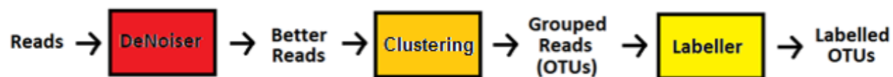
Figure 1.1: An example metagenomics analysis pipeline. Each stage gets executed sequentially, with the output of a specific stage serving as input to a later stage of the pipeline.
